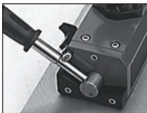
The lifter is in the ON position
