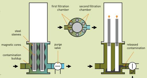
**In use** Contamination is attracted to the sleeve of the cores. Cleaned fluid is re-circulated.
