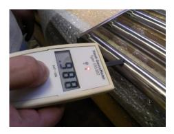
A green LED shows a south pole, a red LED the north pole (2). Measurements are always taken by laying the device with the sensor gently "from above" onto the magnetic pole under investigation. It is essential to follow this convention as otherwise exactly the opposite polarity will be displayed.
